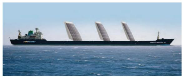
Figure 3.16 An image of a combination of solar and wind energy from Solar Sailor
