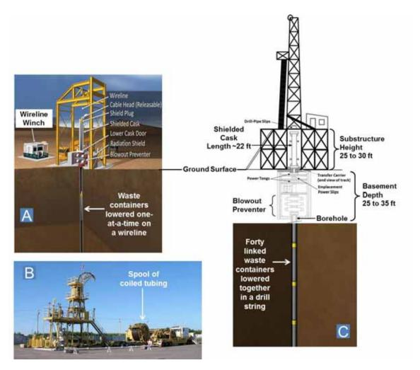
Figure 2. Comparison of deep borehole emplacement modes: (A) wireline, (B) coiled tubing, and (C) drill-string
