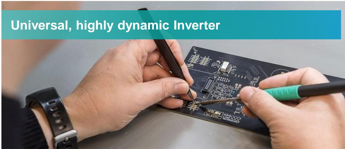
Tapas, a new inverter developed by Corporate Technology, is 10 to 50 times more dynamic than conventional systems, and more compact. This makes it especially well-suited for robots that require great precision at high speeds. However, there are many more potential application fields. The inverter could, for example, be used in wireless charging, 3D printing or LED and laser technology.
