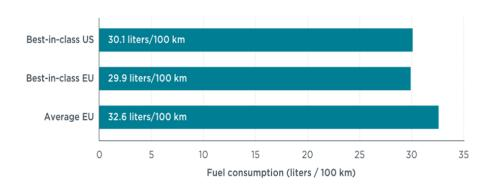
research shows this is not true. Independent on road tests prove that the fuel consumption of US trucks today is comparable to EU trucks (see image).\*\* On top of this the US has introduced a 2027 standards that will make class 8 trucks (comparable to VECTO categories 5 and 10) 27% more fuel efficient compared to 2017 models.\*\*
